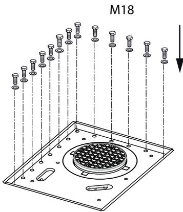
**NOTE WELL: IT IS RECOMMENDED THAT ALL THE FIXING SCREWS BE LUBRICATED BY GREASE**
