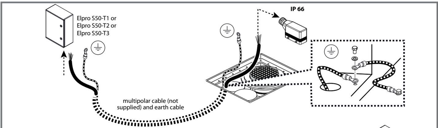
**!** Connections to the terminals of Elpro S50-T1 or Elpro S50-T2 or Elpro S50-T3 controllers (by cable type BUT FLESSIBILE FG 7OR 12x1,5 mm<sup>2</sup>) Earth cable size based on the characteristics of the place of installation.
