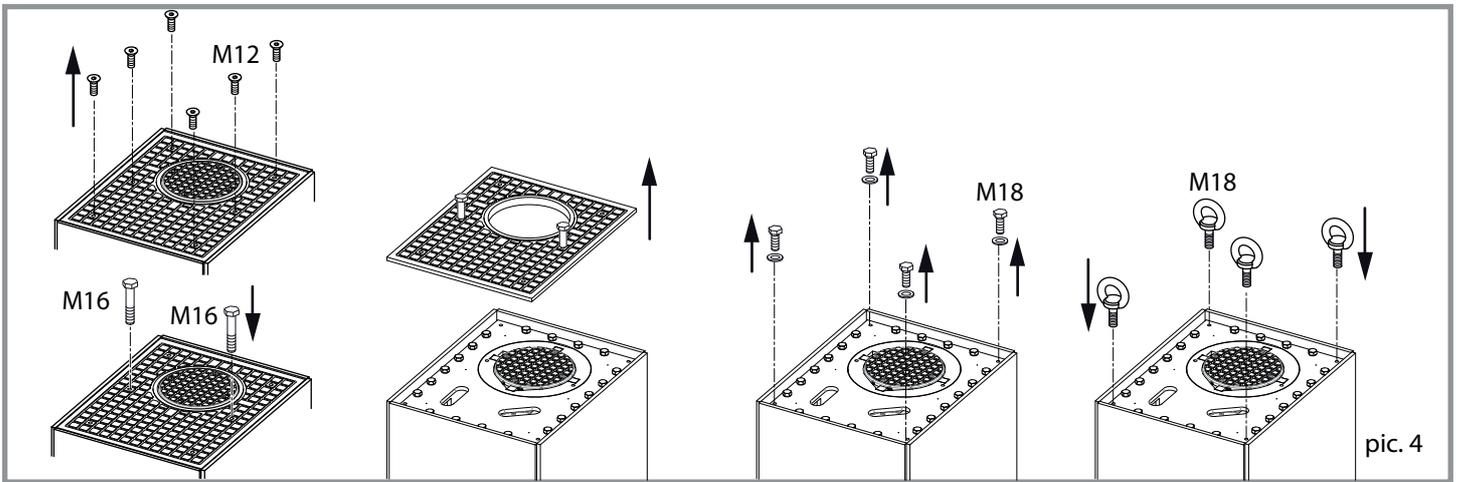
Position the bollard as indicated in the picture, and use a level to make sure it is in axis.
