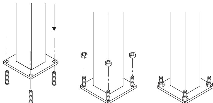
Mount the stainless steel square section post on to the fixing block by means of the useful handling ring fitted to it; eventually tighten the four stainless steel M16 blind nuts.
